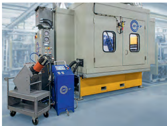
Fig. 1 • Commercial down-stream injection cold spray system (Source: CenterLine Windsor Ltd.).
