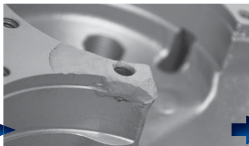
2. Spray Quickly coat. Fill damaged areas as much as one inch.
